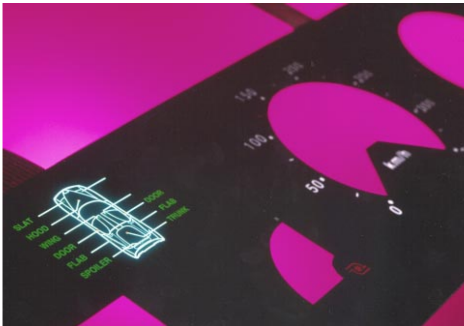
EL Application – Automotive dashboard for Alfa Romeo Scighera. Thin, even illumination is achieved
